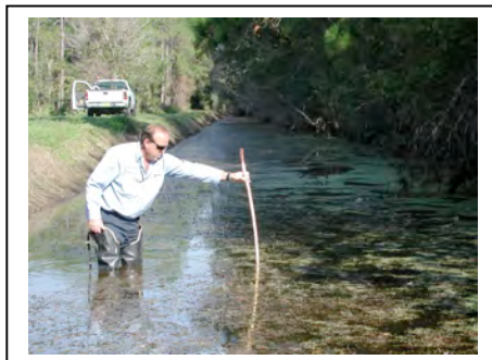
Fig. 3: Rick Swift Measuring Acre-Foot of Drainage Ditch for Rate of Application Determination
